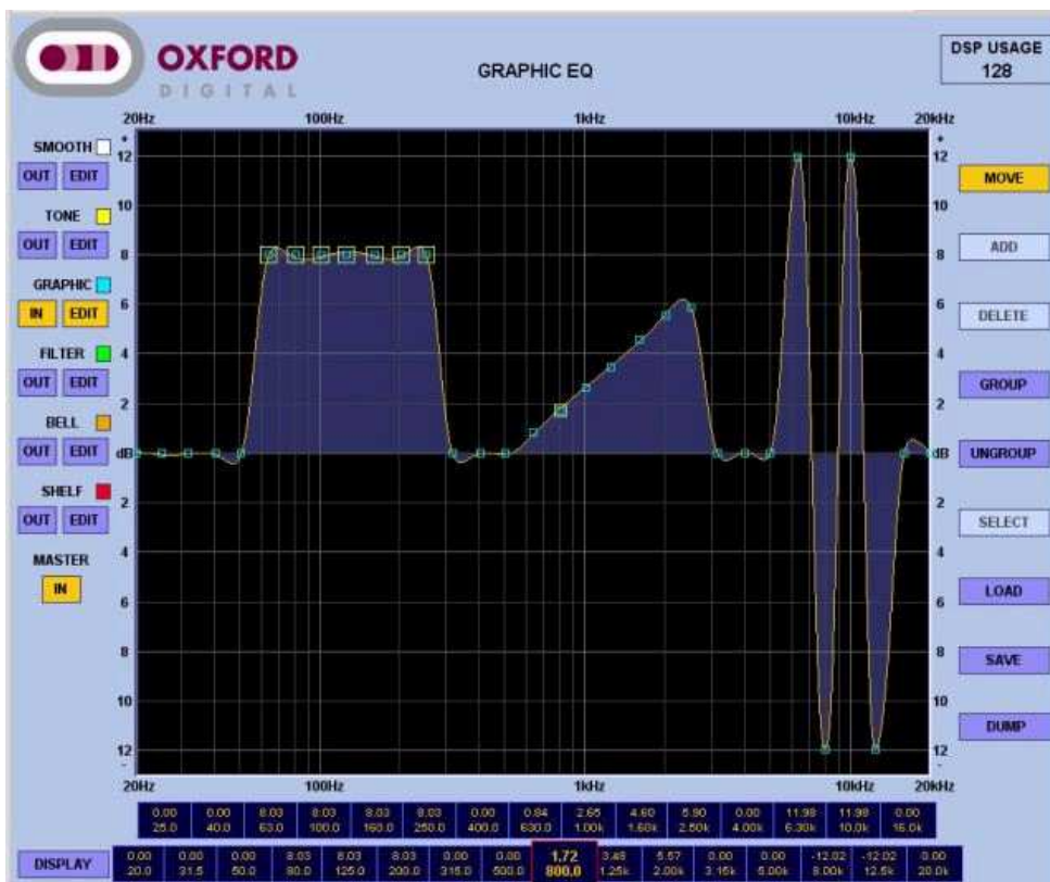
Fig. 6 Example of response of the New Graphic EQ (Yellow line shows actual response)
